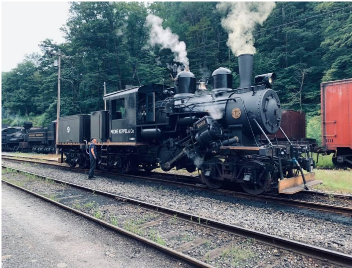
Cass Scenic Railroad Climax No. 9 steams in 2019 after a restoration. The three-truck model previously belonged to Moore-Keppel & Co. Cass Scenic Railroad photo
